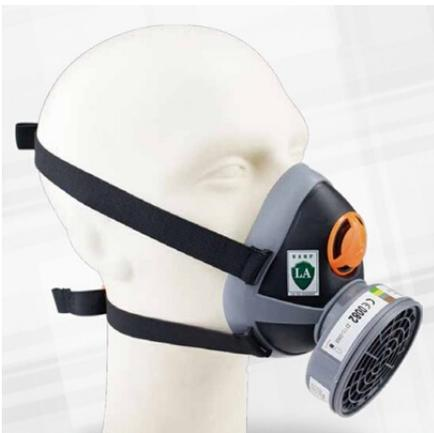
**Description:** Half mask in PP and TPE equipped with an adjustable elastic head harness in Dacron and Lactoprene and an exhalation valve in silicone. The half mask is equipped with one special bayonet connector including an inhalation valve in silicone (detailed description in EC type examination report 15.7.031.001)
